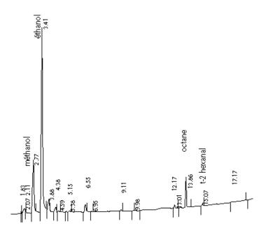
Figure 7. HS/GC - Chromatogram of an extra virgin olive oil.
