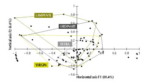
Figure 4. Quality control of VOO - Electronic nose results (PCA). Product mapping, 78 oils, 12 MOS.
