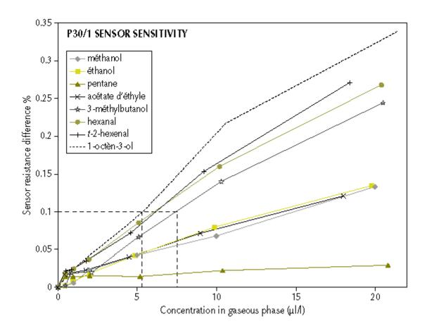
Figure 9. EN - Sensitivity to some volatiles in VOO.
