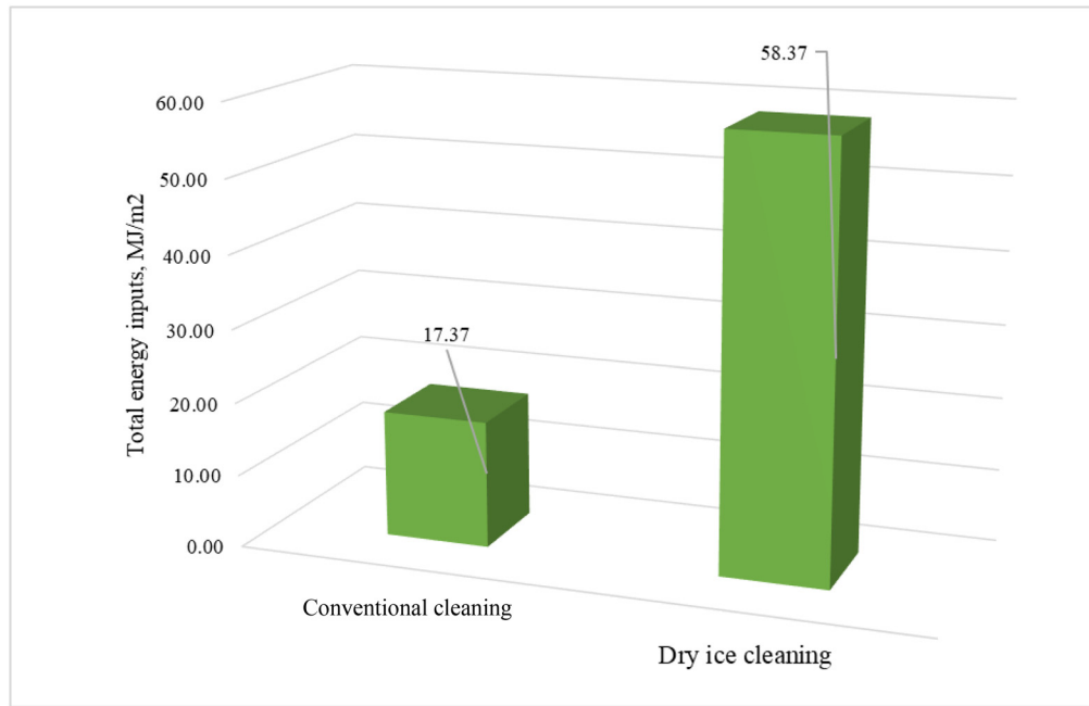
Fig. 5. Comparison of the total energy inputs for conventional and dry ice cleaning methods.
