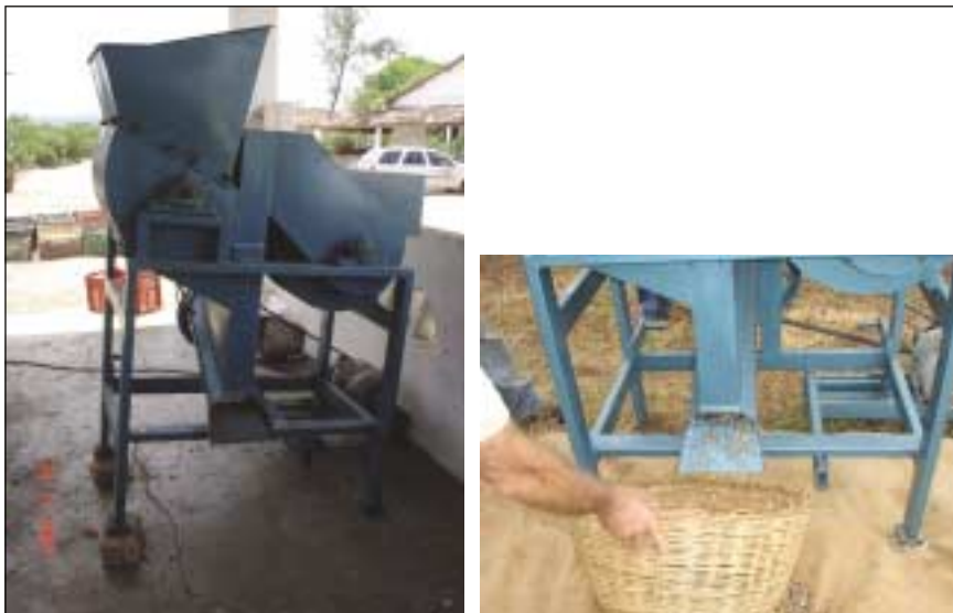
Figure 3. Castor Seeds treatment: the equipment permits deshelling 85% of the fruits, with an operational capacity of 650 kg seeds per hour.
